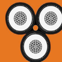
**TRIPLEX FORMATION IS QUICKER TO INSTALL COMPARED TO 3x SINGLE CORE CABLES FOR THREE-PHASE POWER**
