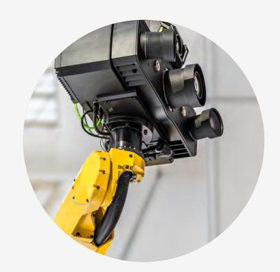
Machine vision refers to the capability to perceive and comprehend the industrial environment using cameras, analog-to-digital (ADC) conversion and digital signal processing (DSP). These technologies allow computers to understand the processes that are taking place so necessary measures can be taken to enhance employee safety and productivity.
