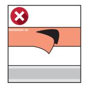
Don't attempt to lift cable drums without inserting the forklift tynes fully under both flanges as they can damage the cable, making it unserviceable. Do not attempt to lift drums by the flange or to lift drums into the upright (correct) position by lifting the top flanges as it may break the flange away from the drum barrel. The drum will then be undeliverable. Use a length of steel pipe through the centre of the drum to provide leverage and control.
