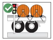
Ensure drums are restrained to restrict movement during sudden stop/starts.
