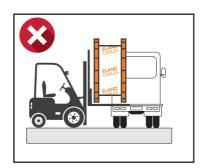
Do not use the forklift tynes to push cable drums sideways on a truck, tray, or direct on the ground as damage to the flanges can result in the drum being unacceptable to customers.
