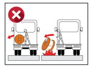
Do not roll cable drums from the back of a delivery truck to the ground as the resulting flange damage will be unacceptable to the customer as the cable will not be able to be rolled off the drum and the drum will need to be returned.
