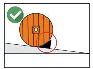
When placing drums on an uneven surface be prepared to check drums against rolling and chock if required.
