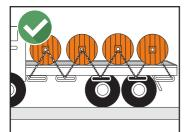
Heavy drums should be chained appropriately for transit, with protection from the chain rubbers for the spindle hole in the centre of the drum. Under no circumstances are drums to be transported on their side.
